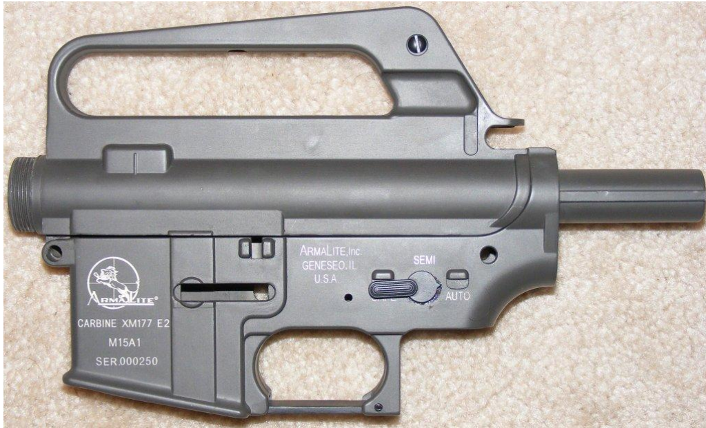
Image 3: The AR-15 style of firearm is marked on the lower receiver with the factory serial number in accordance with USA federal legislation.
